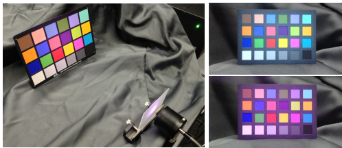
Figure 1: Our setup (left) and the MacBeth Color Checker illuminated by “basis lights” (right). We are able to fully capture scene spectral reflectance despite the amount of ambient light shown here.
